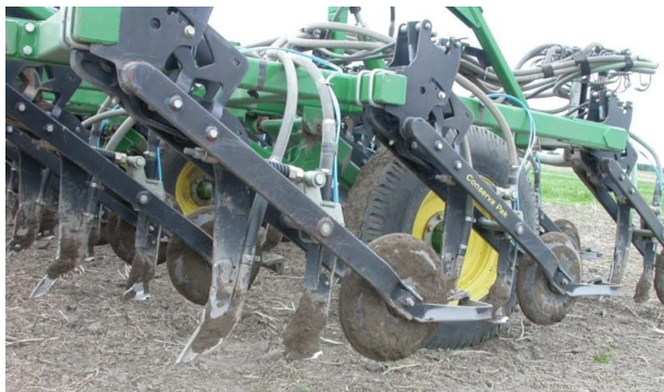
Openers on Conservapak seed drill place fertilizer 2” below & between 2 paired seed rows.
