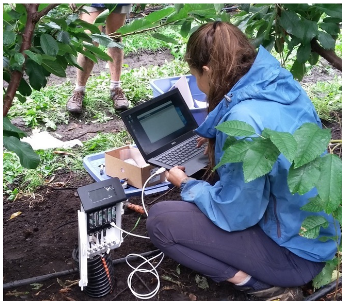
PhD student Elizabeth Houghton downloading soil moisture content measurements from a cherry orchard experiencing different levels of postharvest deficit irrigation
