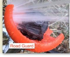
A **full-circle** sprinkler with a **6 gpm** nozzle applies 0.24"/hr.
