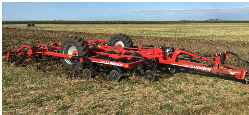
A Horsch high speed tillage disc working up perennial forage stand in the fall after being sprayed out.
