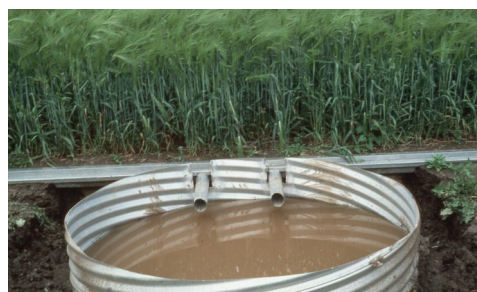
Tank full of water & soil after a summer storm event during the first season at the erosion plots in South Dawson.
